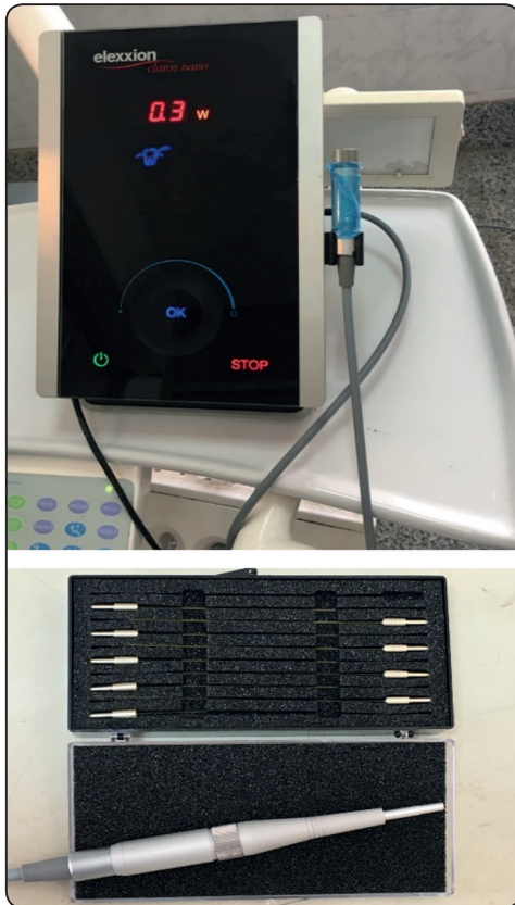
Fig. (1) Ga Al As diode laser (elexxion claros nano compact class IV dental, Radolfzell, Germany) and 200 \mu m fiberoptic.
